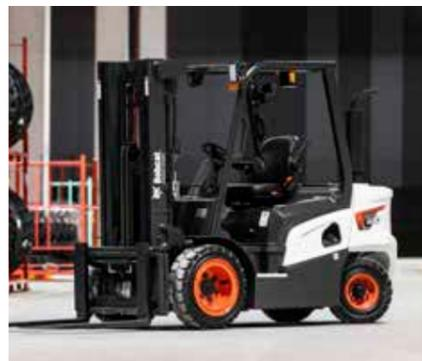
The use of a new U-joint powertrain and oil-cooled disc brakes helps minimize noise and vibration to 77 dBA at the operator's ears.
